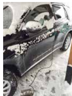
Supplying electricity from the Outlander PHEV
